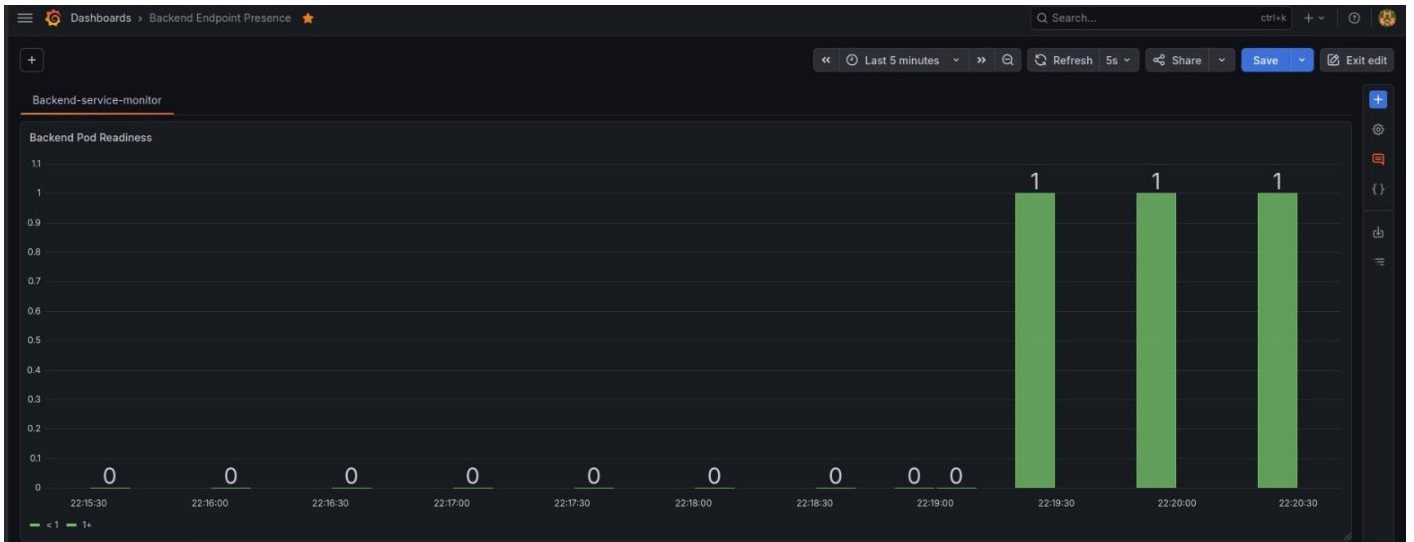
Fig 6.4.2: Grafana dashboard showing pod becoming unhealthy due to CPU-intensive event loop blocking
